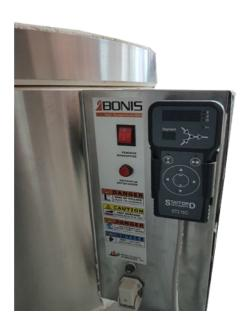
Plug the Controller socket into the socket on the electrical panel of the kiln and secure it with the shutter.
