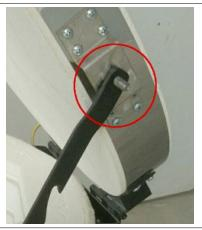
Remove the bar from the bottom of the support base
