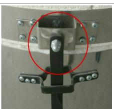
Open the lid and remove the bar from the screw that supports it
